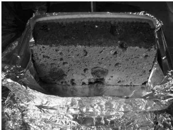
Fig. 1. Experimental setting for the diffusion test of Ethyl Silicate.
